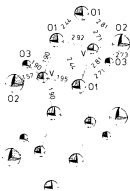
Fig. 2. The zigzag string of VO_5 square pyramids. The thermal ellipsoids are drawn at 90% probability.
